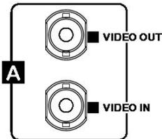
Each monitor has a composite video input, with a loop-through output (5). The video input can be PAL or NTSC, the TLM-433 will automatically detect the video standard.
