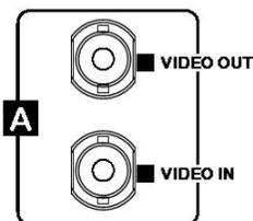
Each monitor has a composite video input (1), with a loop-through output. The video input can be PAL or NTSC, the TLM-433 will automatically detect the video standard.
