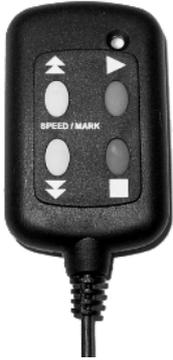
Before you are able to use the wired remote you must first turn on the remote control feature within the prompter software. The remote plugs into the headphone jack on the smart phone. Ensure the remote jack has a good connection with the phone socket. It may be necessary to remove the phone from any 3<sup>rd</sup> party protective skin before the phone is fitted to the prompter hood cradle.
