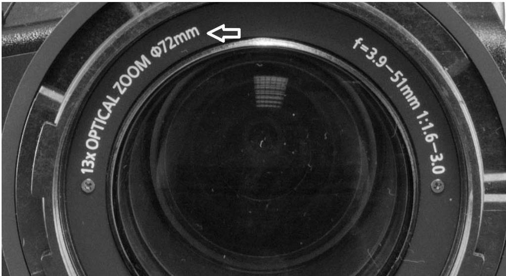
The first thing to find out when using this prompter kit is the diameter size of the lens ring on your chosen camera. Usually this size is printed on the camera lens itself and it can also be found in the camera's manual too. To help you, DataVideo has supplied a variety of rings which are compatible with the Prompter Hood and some of the standard size camera lenses.
