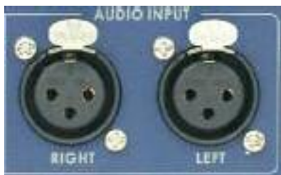
Balanced Audio Input Supports two channels XLR Balanced Audio Input
