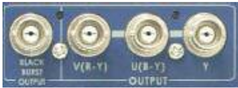
Component Video Y, U, V with Black Burst output terminal for video monitoring
